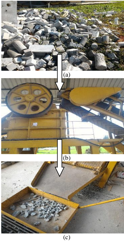
Fig. 1 Process of Obtaining RCA; (a) C&D Wastes;(b) Jaw Crusher ; (c) Sieving[13]
