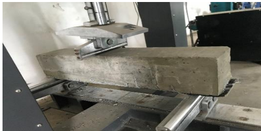
Figure 4 Beam wrapped Bottom
