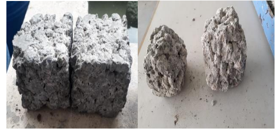
Fig.4 showing the variation in specimens of PC mix before and after abrasion
