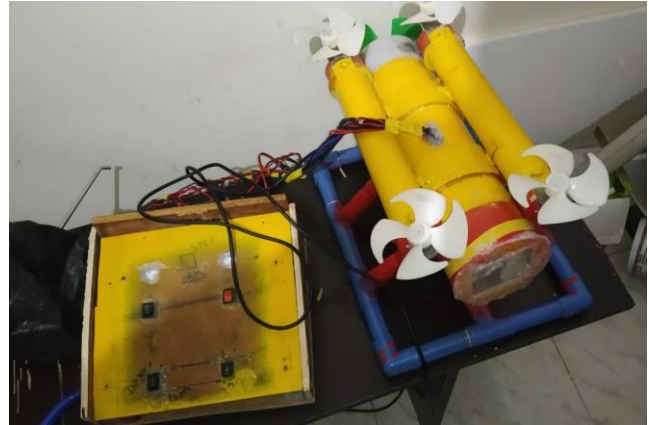
Fig-6: Fabrication of underwater ROV
