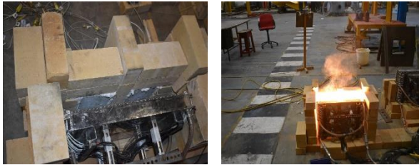
Fig. 3. Experimental set up for Un-coated and Coated samples M30 and M40 blocks coated with 2mm and 4mm thickness of coating were tested.
