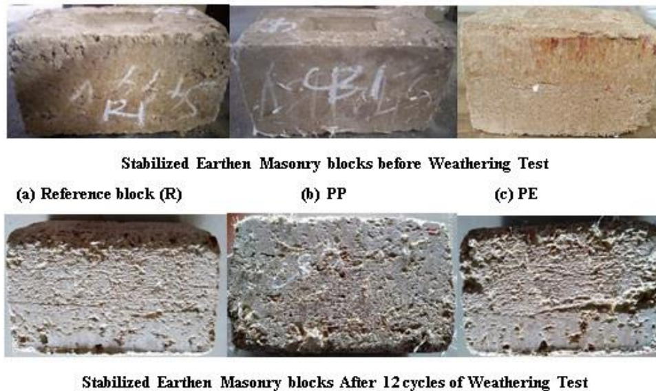
Fig.5. Stabilized lateritic soil blocks before and after weathering test
