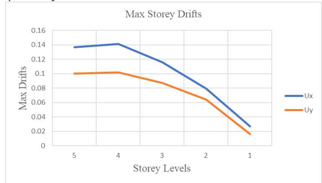
Figure 17: Graph representing the maximum storey Drift in X and Y direction
