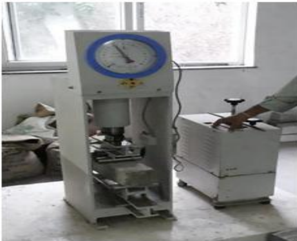
Fig. 1 laboratory set up for flexural study [10]
