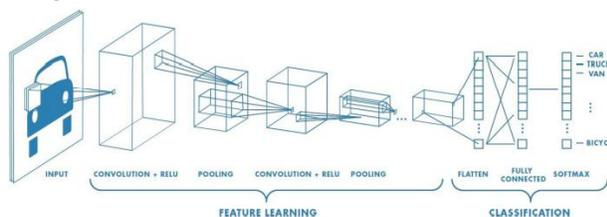
Fig. 1 Architecture of Convolutional Neural Network
