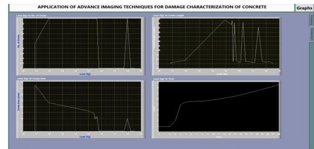
Fig. 5 a) Load vs Number of Cracks, b) Load vs Crack Length, c) Load vs Area of Cracks and d) Load vs Time
