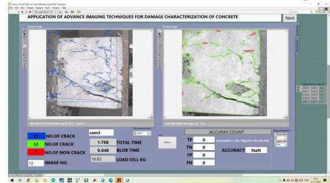
Fig. 4 Concrete Crack Detection Model Result
