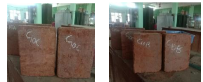
Image 4: Before efflorescence test of stabilized adobe block
