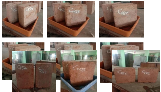
Image 4: Before efflorescence test of stabilized adobe block
