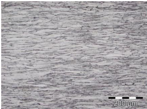
Fig-8: Optical microstructure of Cold rolled-Unannealed IF steel sheet X200
