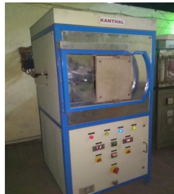
Fig-4: Experimental set-up (a) Rolling of IF grade steel at Experimental Rolling mill, RDCIS; (b) Muffle furnace for annealing, Kanthal Make.
