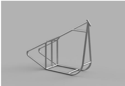
Fig (2): Aluminium 7075 chassis
