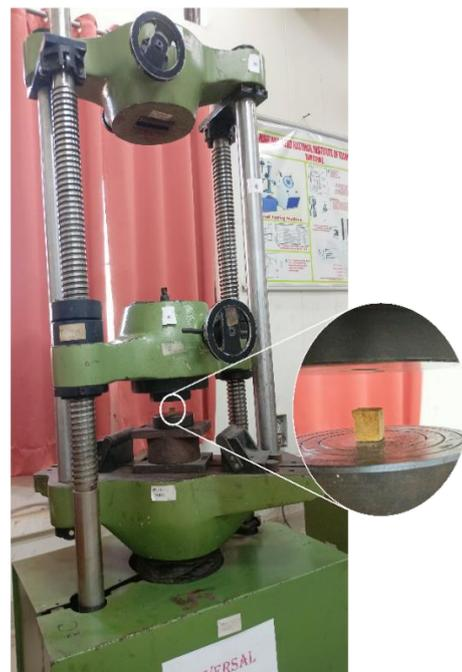
**Figure 6: Sample placed in a Hydraulic Press**
