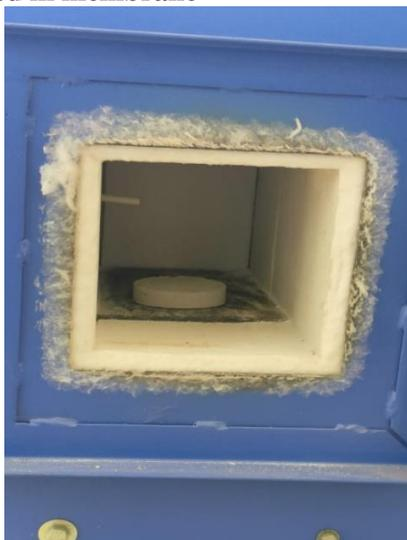
**Figure 2: Sintering of membrane in muffle furnace**
