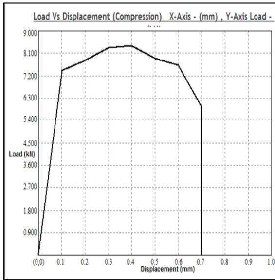
**Figure 7[a]: Membrane S1, Yield Load(kN):5.92 Yield Stress (MPa):26.311**
