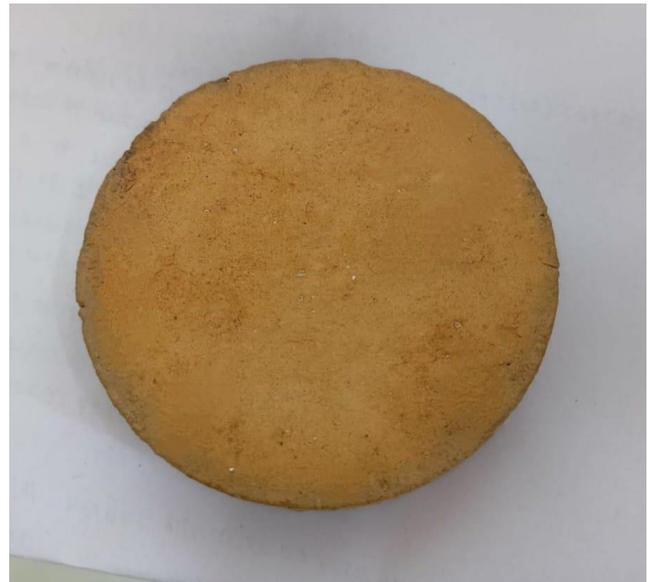
**Figure 3: Ceramic Membrane after sintering in muffle furnace**
