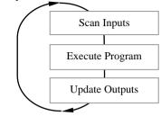
*The Response time = Input Response Time + Program Execution Time + Output Response Time* Generally, the PLC Program cycle should be less than 150 ms.
