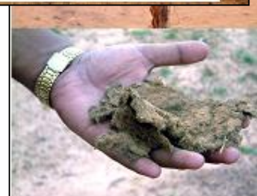
Figure 5: The decomposed status of the fibre after 1 monsoon.
