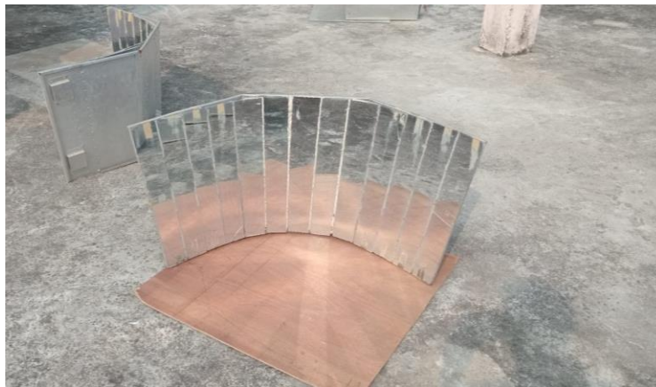
Photo: 13 segment reflector reflection patterns as shown in above picture at 09:30 am on 17 th January 2025.
