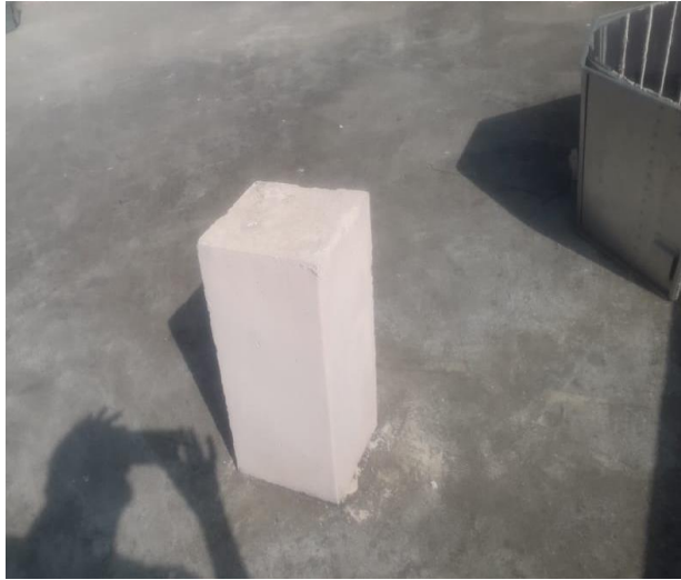
Photo: Sun rays falling on concrete beam 2 sides and top of the beam
