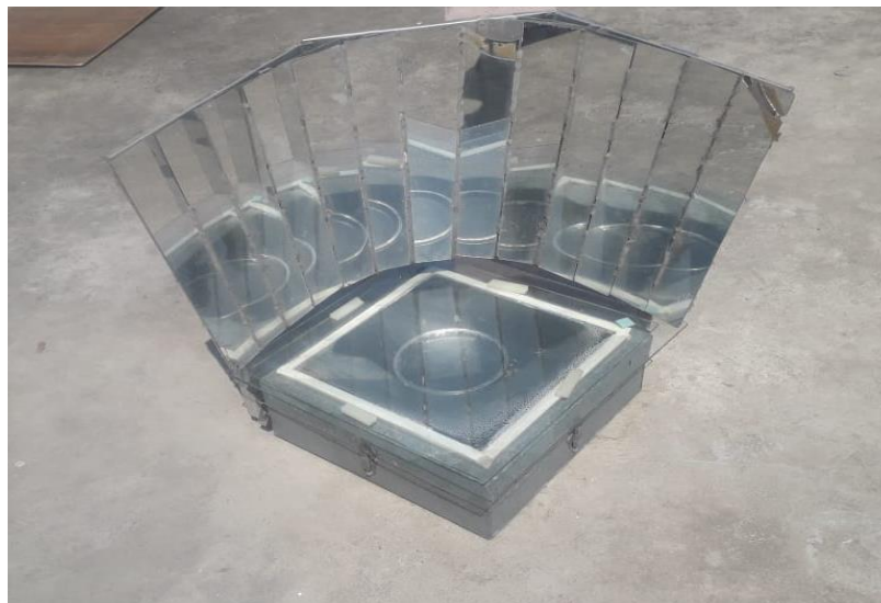
Photo: Box type solar cooker assembly with 13 segments reflector picture after completion of boiling water droplets formed.
