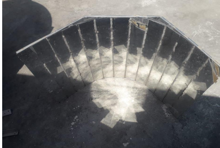
Photo: 13 segment reflector reflection patterns as shown in above picture at 12:00 pm noon on 17 th January 2025.
