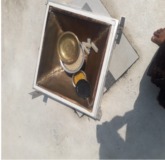
Fig-3: Dal & rice boiled condition above figure
