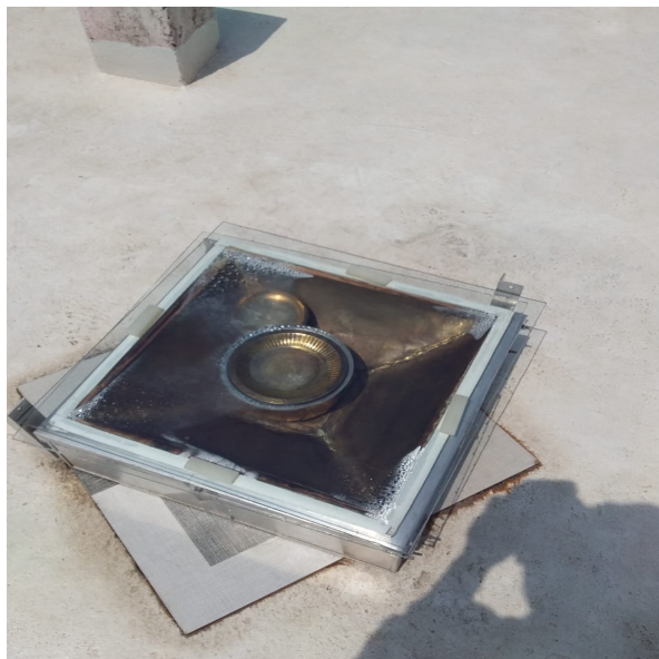
Fig-2: Brass utensil - Steam condensing on bottom cover glass kept in brass trough rice & Dal after boiling
