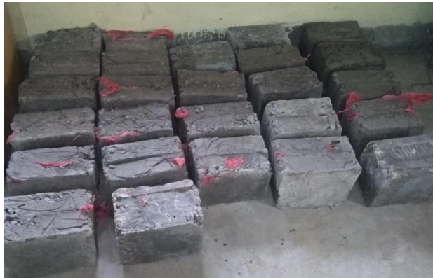
Fig. 4: RCA concrete block
