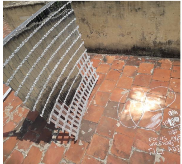
Fig. 11 Spherical segment reflector with slight distributed focus
