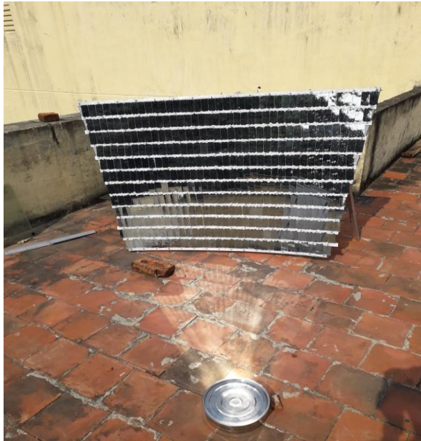
Fig. 8 Paraboloid segment as hood (area) 1.17 mt square As it kept part tilted tested for concentration/focus observation the focus.
