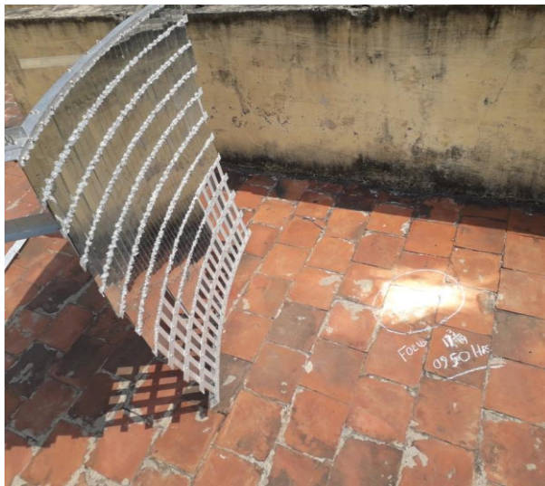
Fig. 8 Paraboloid segment as hood (area) 1.17 mt square As it kept part tilted tested for concentration/focus observation the focus.
